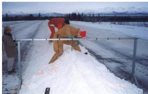
FIGURE A4 - Measuring the Windrow Using a Gantry When Employing the Constructed Windrow
